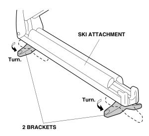
4. Using a wrench, install the ski attachment to the front crossbar with four bolts, four collars, and two brackets.
